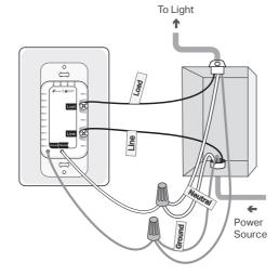
5 Line up the dimmer switch with the mounting holes. Secure it with screw mounting holes. Secure it with screws.
