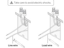
2) Turn off the circuit breaker. Label the Line and Load wires.
